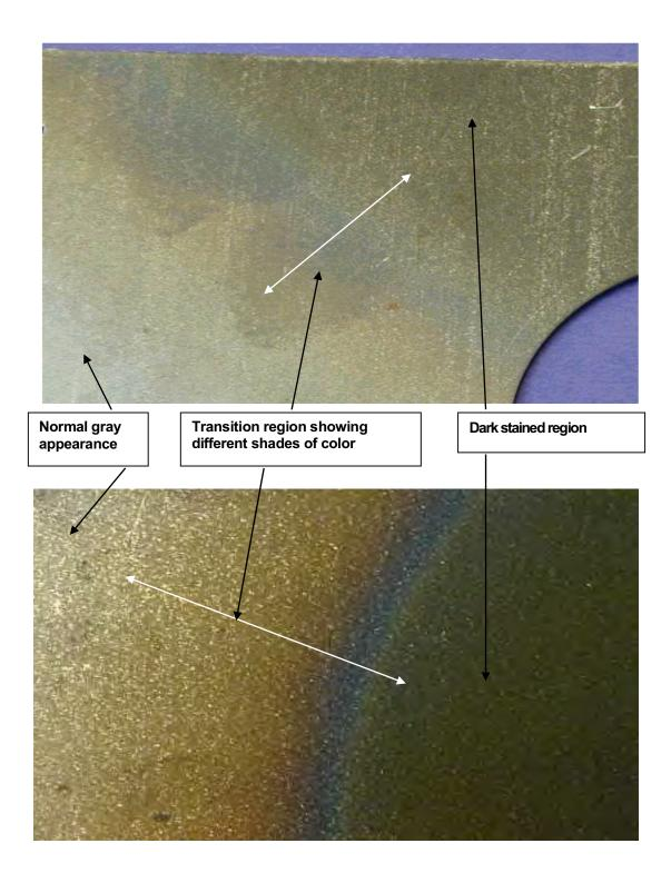
Figure 2: Dark stains on galvannealed steel sheet
