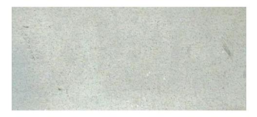
Figure 1: Normal appearance of galvannealed steel sheet
